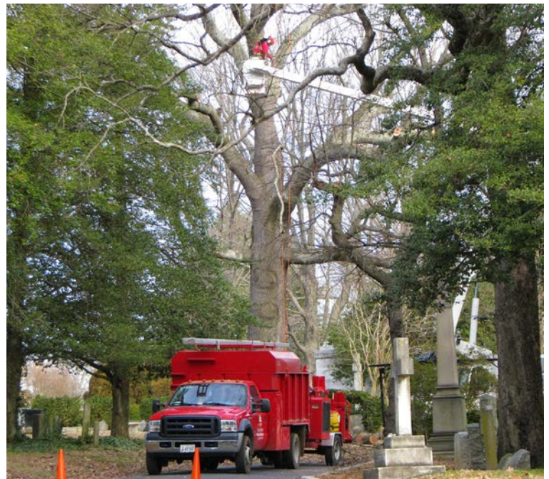
A bucket truck can reach as high as 65 feet.
