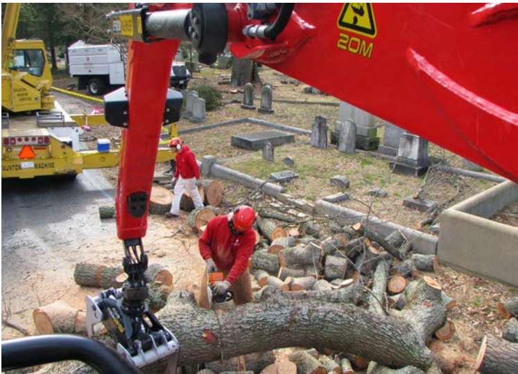
A grapple log loader (made in Austria) is used to lift and load logs into a truck.
